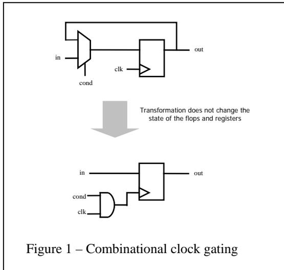
Since combinational clock gated flops maintain a one to one state mapping with the original RTL, Combinational Equivalence Checking Tools can be used for functional verification. This makes verification simple to setup and comprehensive. On the other hand because switching activity is eliminated only when data is not changing, the actual power savings is limited. In typical designs, combinational clock gating can reduce dynamic power by about 5%-10%.
