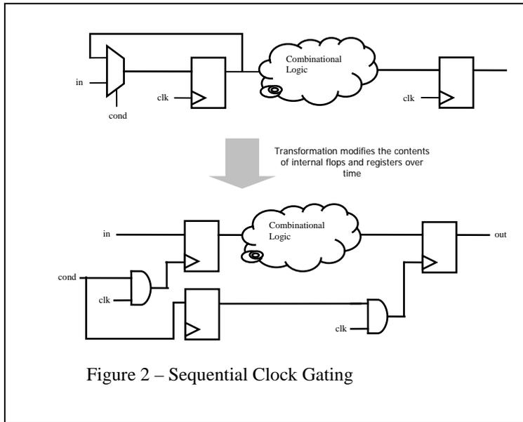
Sequential clock gating is a multi-cycle optimization with multiple implementation tradeoffs and RTL modifications. Consequently there is a greater demand on functional verification resources. On the other hand sequential clock gating can save significant power, typically reducing switching activity by 15-25% on a given block.
