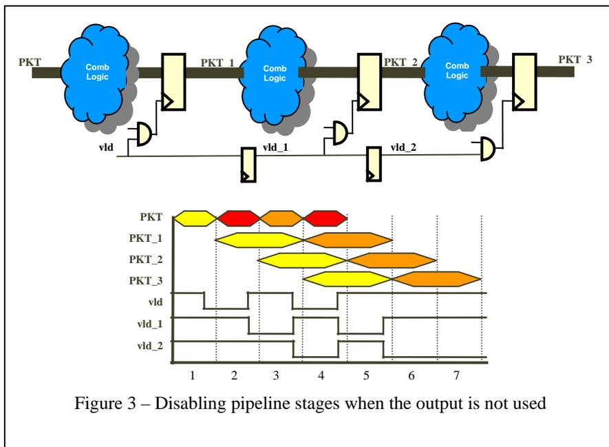
Since this transformation is a sequential RTL change, it cannot be verified with combinational equivalence checking tools. Previous projects showed that simulation regressions are biased towards testing active states in the design, whereas this transformation takes advantage inactive “don’t care” states. With clock gating changes there is always a question about test coverage because it is difficult to test for all combinations of gating states and “don’t care” assumptions.
